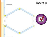
Insert #6 x  $1\frac{1}{2}$ " flat head screws about 8" up from the floor and 8" down from the track on both sides.
