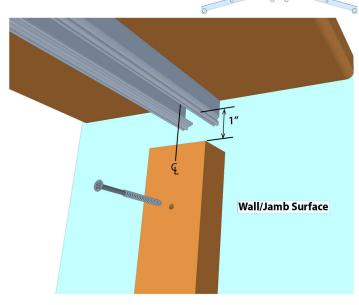
Push the door over the post. The post will snugly fit between the mounting panel flaps. Screw the mounting panel flaps to the post using the provided #6 x  $1\frac{1}{2}$  flat head screws. Place a screw about 6" from the top and bottom of the post and 2 additional screws equal distances between the first 2 screws. Repeat anchoring the 2nd flap being sure to slightly offset the screws so they won't meet in the middle of the post.
