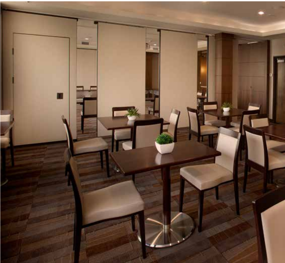
Panels nest deeply and seal tightly to create an acoustic barrier with a rating of 56 STC - the highest in the industry.
